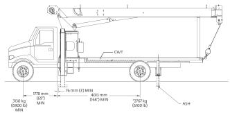
This configuration is the least expensive method for the Model 571E2. This mount, with the crane mounted behind the cab, requires the least weight of all mounts for stability; thus, you can haul larger payloads on your truck. It requires standard subbase and rear (ASH) stabilizers.
