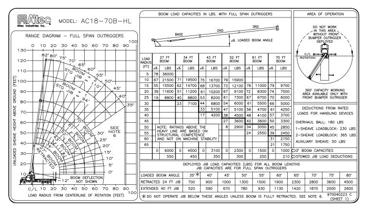
Note 1: When jib is erected, boom must be fully retracted before lowering below minimum boom with jib angles. Retracted boom with jib has no lifting capacity below a 50° angle with full span outriggers and below a 65° angle not shown on jib load rating chart.
